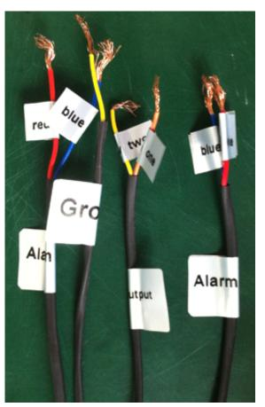
You will see the camera with alarm wires as below, each wire with a label of alarm input and output, just connect them to your alarm devices, You can see the labels marked one / two / three / four, these means they are alarm in 1...alarm in 4, the grounding wire is for all alarm input wires use together.
